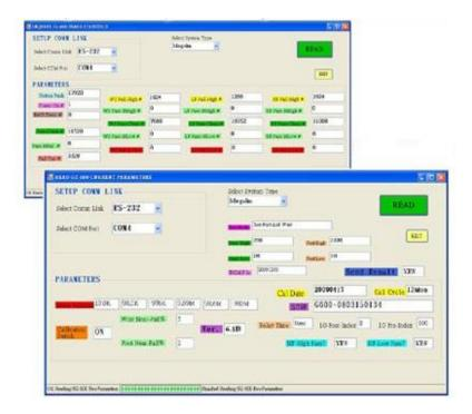
This stand-alone program designed for the hardware management of the Captain GREEN Series defensive ESD testers. It uses the RS-232 serial port to communicate with the tester hardware for data exchange. The main functions are to read the tester's internal control parameters and usage statistics and to set new control parameters.
